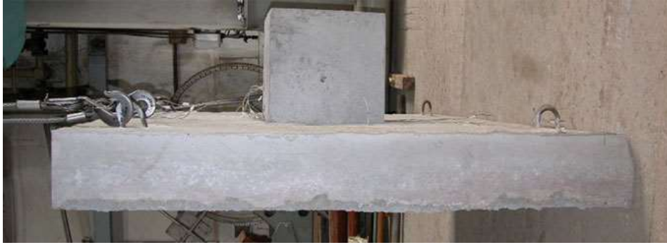
Fig. 2 Prototype in [7] after punching failure. Side view
